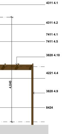
4311 4.1 0.40MM CORRUGATE PROFILE METAL ROOFING [refer spec]
