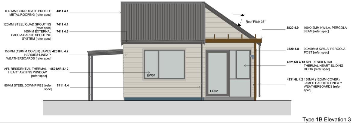
0.40MM CORRUGATE 4311 4.1 PROFILE METAL ROOFING [refer spec] 125MM STEEL QUAD 7411 4.1 SPOUTING [refer spec] 165MM EXTERNAL 7411 4.6 -FASCIA/BARGE SPOUTING SYSTEM [refer spec] ROOFING [refer spec] ■ੑੑਗ਼੶ੑੑੑਸ਼ੑਗ਼ਗ਼ਗ਼ਗ਼ਗ਼ਗ਼ਗ਼ਗ਼ਗ਼ਗ਼ਗ਼ਗ਼ਗ਼ਗ਼ਗ਼ਗ਼ਗ਼ਗ਼ਗ਼ਗ਼ਗ਼ 150MM (120MM COVER) **4231HL 4.2** JAMES HARDIE® LINEA™ WEATHERBOARDS [refer spec] EW05
