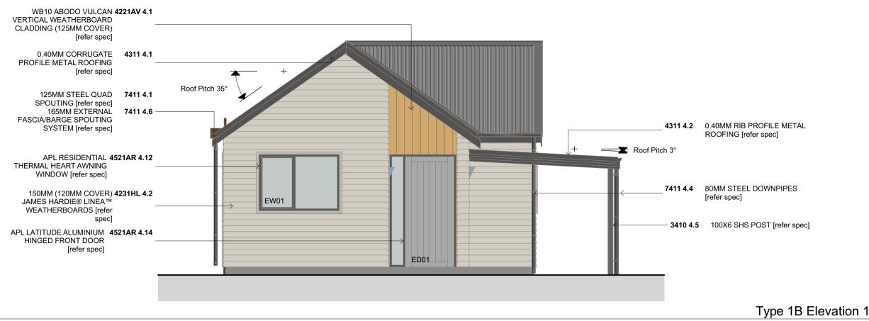
SPOUTING [refer spec] 165MM EXTERNAL 7411 4.6 -FASCIA/BARGE SPOUTING SYSTEM [refer spec]
